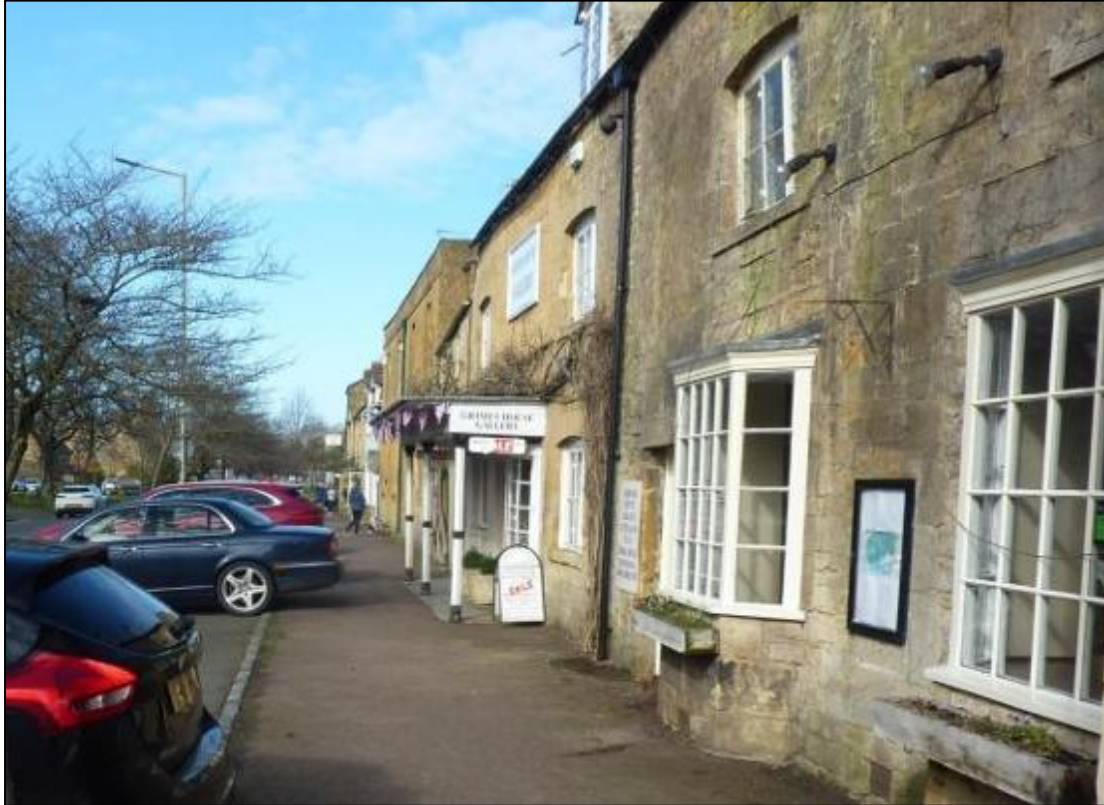
Figure 2-24: Pavement parking overhanging footway
